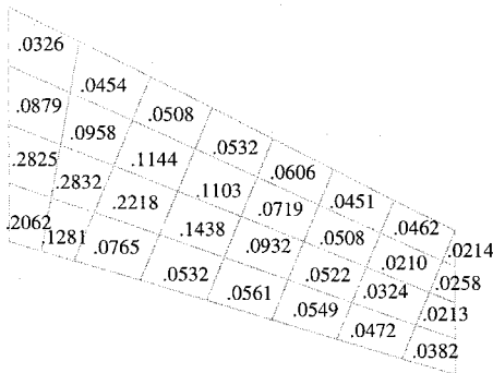
Fig. 11 Thickness distribution for the top and bottom skins -20-deg rotation angle. Stress, size, and aileron effectiveness constraints.
